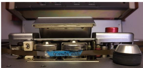
**FIGURE 1.** Example of markings on a tape splice.
